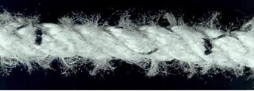
Figure D-55 - UV (Sunlight) Degradation of polypropylene rope
