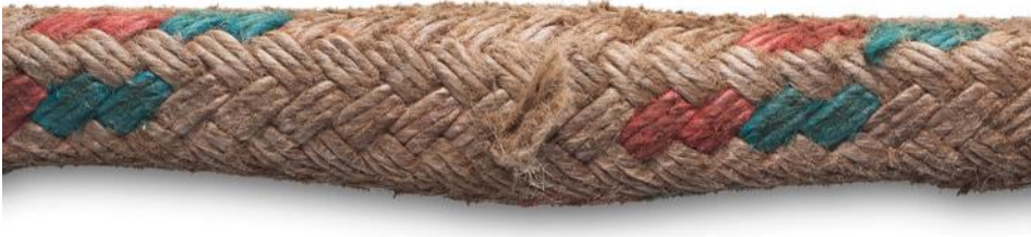
Figure D-47 - Core axially compressed causing winch bumps that can be restored (photo credit: Yale Cordage)
