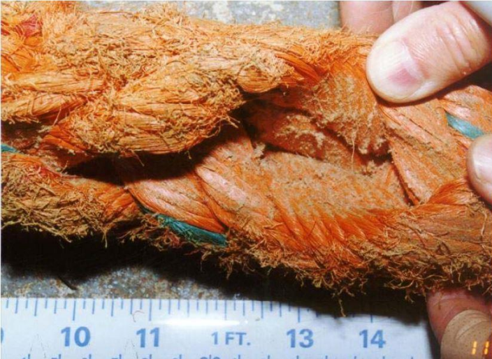
Figure D-5 – 8-strand rope showing internal flattening, abrasion, and fusing. (photo credit: TTI)
