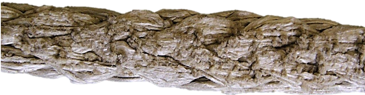
Figure D-16 –Extreme external abrasion wear (photo credit: ISO)
