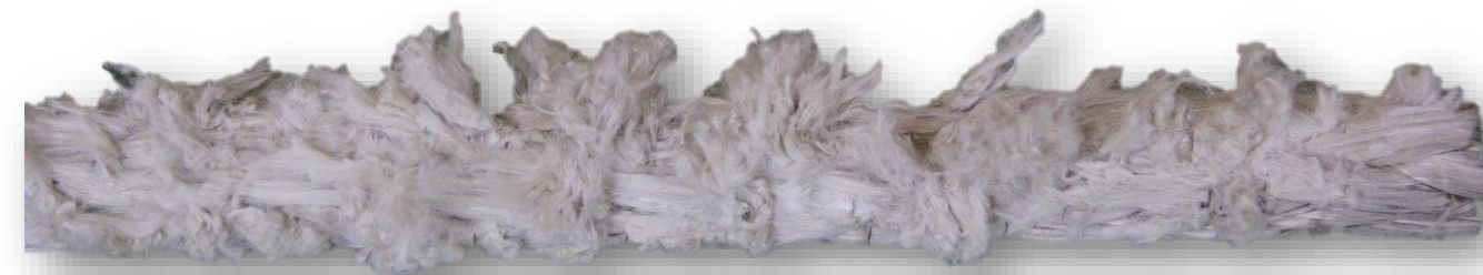
Figure -17 - Extensive external abrasion on a braid (photo credit: ISO)
