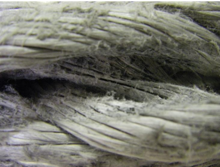
Figure D-6 - Inter-Strand Abrasion (Exposed internal area reveals wear at strand internal contact points)
