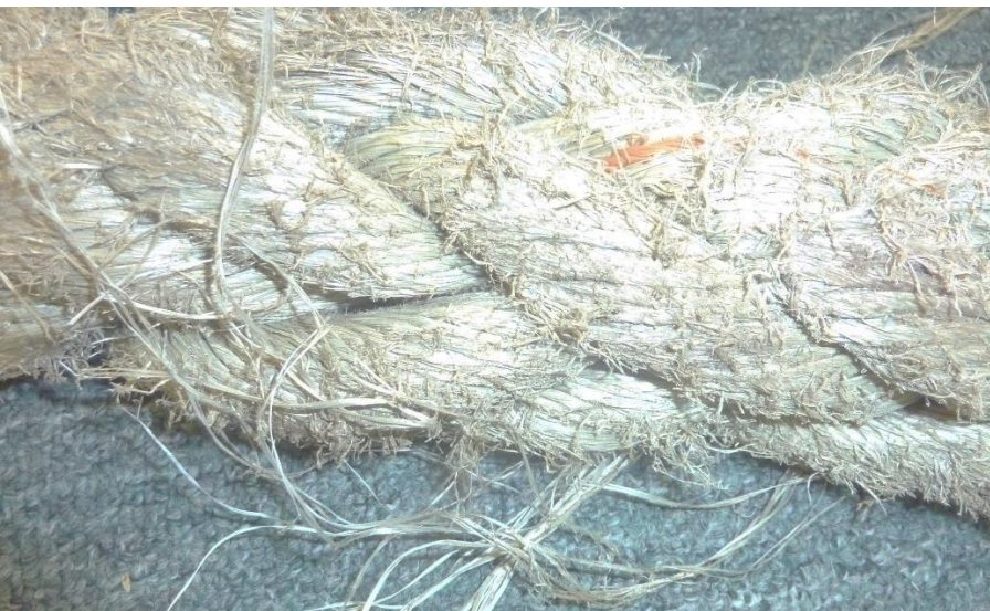
Figure D-57 – Braided rope degraded by sunlight
