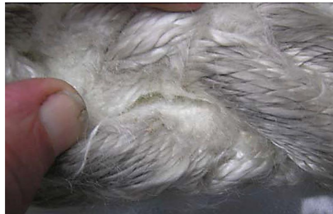
Figure D-8 – 8-strand rope opened to show abrasion between strands.
