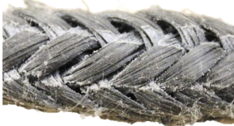
Figure D-7 - Inter-Strand Abrasion (exposed internal area reveals fiber to fiber abrasion at braid crossing points.)
