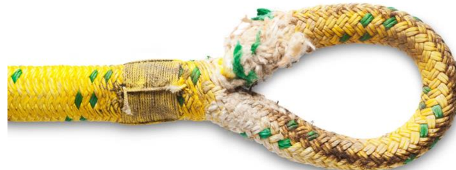
Figure D-43 – Worn-out eye of a balanced double braid (photo credit: Yale Cordage)
