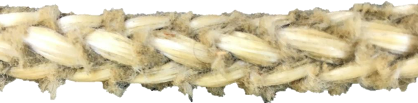
Figure D-56 – 8-strand braided rope degraded by sunlight in need of retiring (photo credit: Teufelberger)
