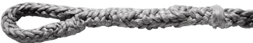
Figure D-41 – Improper splicing of a 12-strand braid
