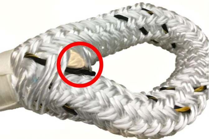
Figure D-42 – Top picture of a properly made splice for reference. Bottom picture is slipped splice on a double braid after tension was applied. Core is exposed and colored warmer. (photo credit: Teufelberger)
