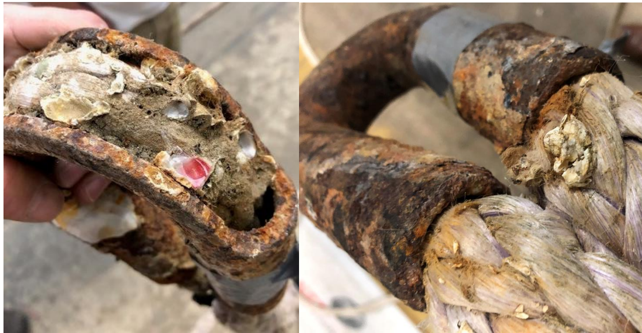
Figure D-46 – Thimble with corrosion and bio-fouling. Both pictures are the same thimble/rope taken from different angles.(photo credit: Cortland Company)
