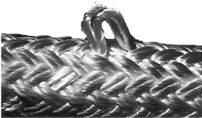
Figure D-33 - Pulled strand in new double braid. Load bearing core is intact.
